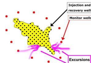
"One of the major problems associated with the in situ mining method is the uncontrolled migration of lixiviant and dissolved constituents such as radionuclides, arsenic, selenium, chromium and lead outside of the production zone. These undesirable lixiviant migrations are known as excursions."<sup>4</sup>
